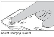
When the battery is fully charged, the charge status LED will glow constant WHITE. Unplug the battery from the charger and press the circular button once, the charger will be ready to charge
